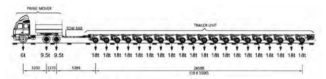
Fig. 6: Typical Axle Arrangement for Special Vehicle
