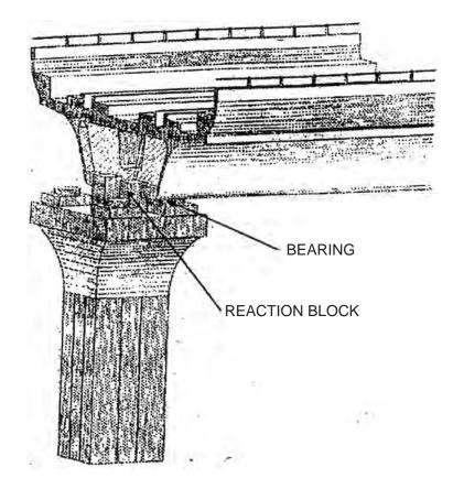
Fig. 21: Example of Seismic Reaction Blocks for Simply Supported Bridges
