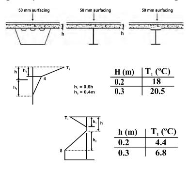
Fig. 16b: Temperature Differences Across Steel and Composite SectionNote : For intermediate slab thickness, T<sub>1</sub> may be interpolated.
