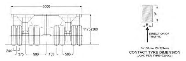
Fig. 6A: Transverse Wheel Spacing of Special Vehicle
