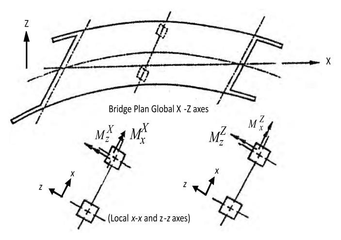
Fig. 18: Combination of Orthogonal Seismic Forces
