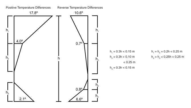
Fig. 16a: Design Temperature Differences for Concrete Bridge Decks
