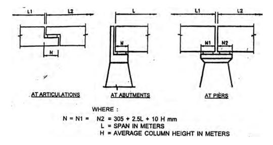
Fig. 22: Minimum Dimension for Support
