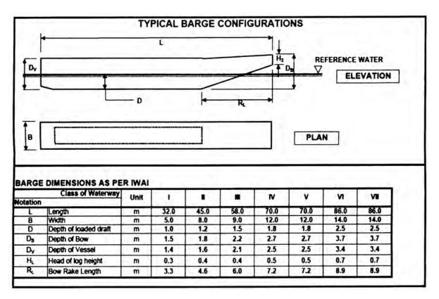
Fig. 23: Typical Barge Dimensions
