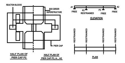
Fig. 20: Example of Seismic Reaction Blocks for Continuous Superstructure
